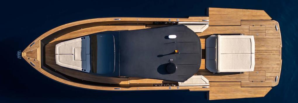
The foldable wings are designed to optimize space on board. When deployed, each wing extends the beam of the boat by more than 0.5 meters, providing additional space for activities and increasing comfort. This innovative design allows for a larger and more versatile area.
